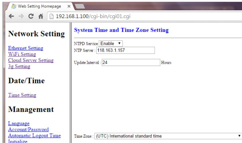
NTPD Service: Enables or disables NTPD (Network Time Protocol Daemon, a service that automatically synchronizes G07's current date and time settings periodically) (**Enable / Disable**). The default option is **Enable**.
