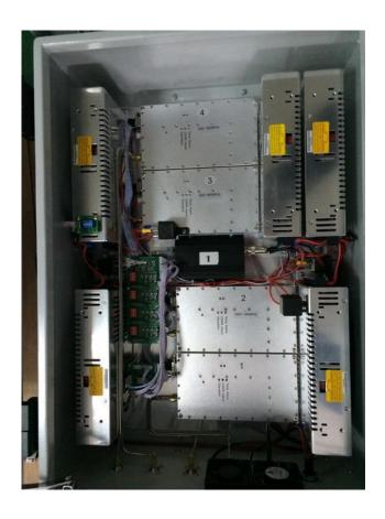
The CT-4030 also houses individual module control units, for controlling jamming at specific frequency bands that are placed in the openings of the chassis casing. You can tell which module control unit handles which frequency band as it includes a Number-Code on the front of the module.
