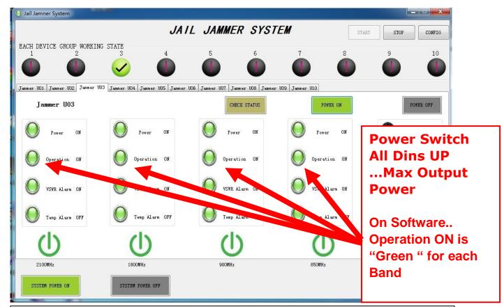
You have now successfully set up the CT-4030 to jam signals. To perform further configurations from a notebook, such as Turn ON/OFF each band, each jammer o the whole jammer system, follow the procedure below for initializing remote control software.
