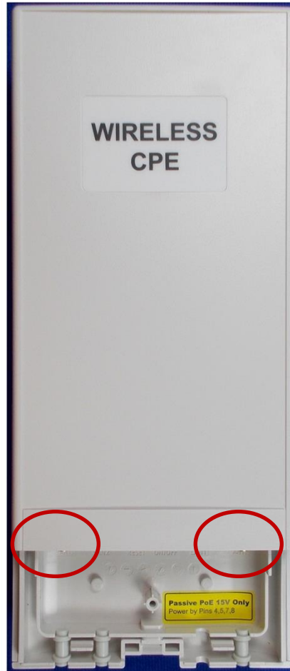
SMA connectors x 2 For antenna external
